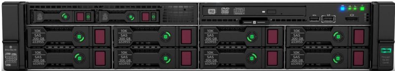
8LFF Chassis with Universal Media + 2SFF
