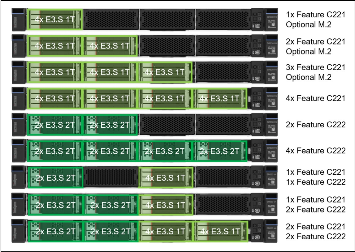
Figure 13. SR630 V4 front drive bay configurations - E3.S drive bays
